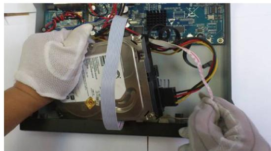
3. Fix the HDD on the bottom plate
